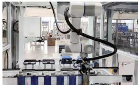
Battery Inspection Loading & Unloading
