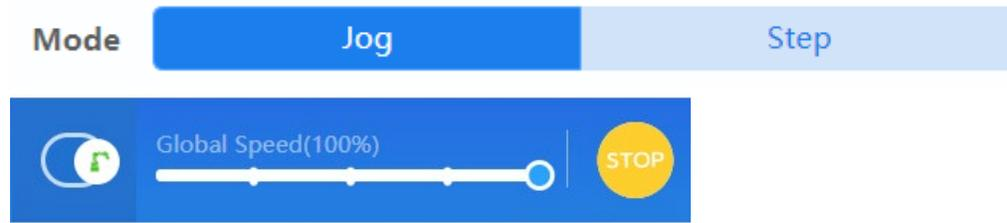
In "Step" mode, the robot will increment the selected distance in mm whenever the user taps a button. For example, the following button configuration would drive the robot 1mm in the x-direction when clicked:
