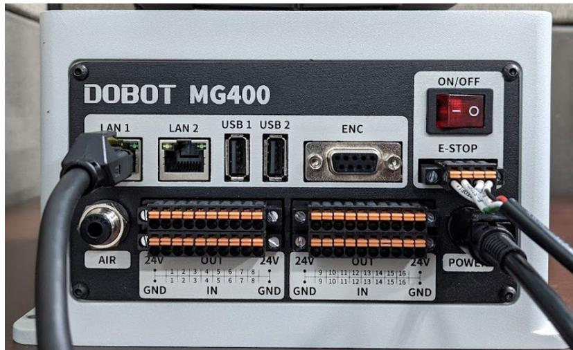
Next, flip the ON/OFF switch to the ON position. The switch LED should turn on, as shown here:
